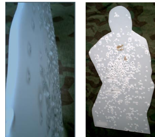
Self-sealing plastic target after 1000 hits
